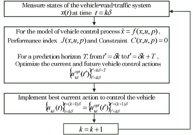
Fig. 3 Model predictive control of a vehicle.
