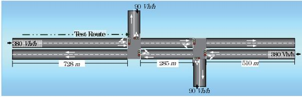
Fig. 6 An image of the test environment, traffics, and route used in AIMSUN NG.
